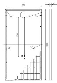
A: 4 x drainage 10\*10 mm B: 8 x ventilation aperture 3\*7 mm C: 8 x mounting hole<sup>4</sup> d = 7 mm D: 2 x earthing d = 2 mm
